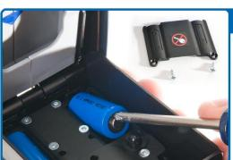
3. Flip the battery cover open and reveal the two batteries.
