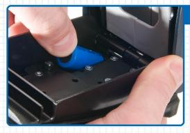
5.Using two NEW CR123A batteries, install each battery into their battery cavity with the positive terminal going in first. The terminals are staggered, so the batteries will be facing different directions.
