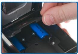
6.Install the battery cover. There are tabs on the bottom of the cover that slide under the hooks directly above and behind the battery cavities. Slide the tabs in under these hooks at an angle and lower the front of the cover down flat.
