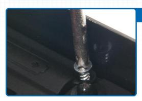
7.Re-install the two battery cover screws with the Phillips head screwdriver.
